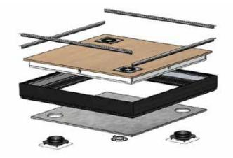
**3c** Screw the wedges under the ceiling.
