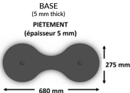
Unique base narrower than the two acoustic screens it accommodates for easier circulation around the Duo 360.
